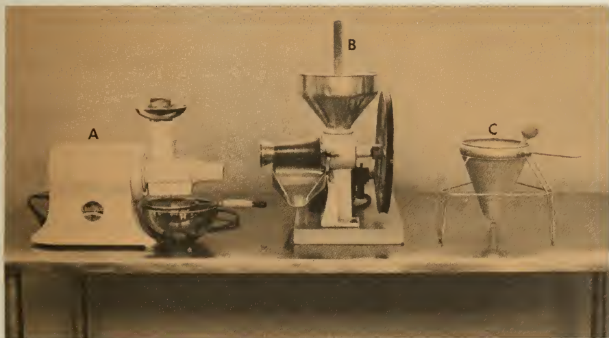
Figure 7. Small juice-extracting units. A and B, Juicers suitable for extracting several gallons of juice for canning or freezing. C. Cone-shaped food press.
